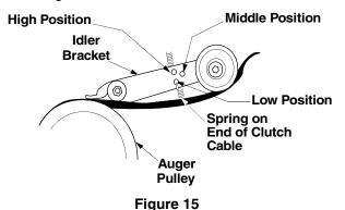
To adjust, move the extension spring on the end of the clutch cable to the next higher adjustment position on the idler bracket assembly. Reassemble belt cover.
